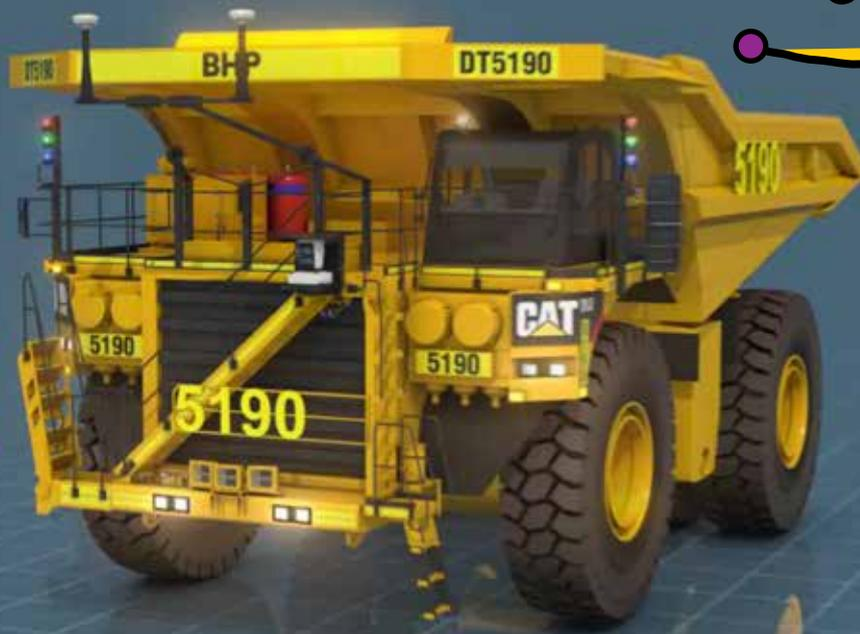
Autonomous trucks may look the same as their counterparts with drivers, but there are more than 7,000 additional parts required to give it the 'eyes and ears' needed to navigate around the mine site.
